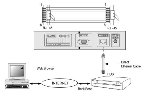
Connected from SNS-110 to PC(Twisted Cable)
